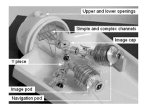
Figure 2: Dexter. Internal Components
